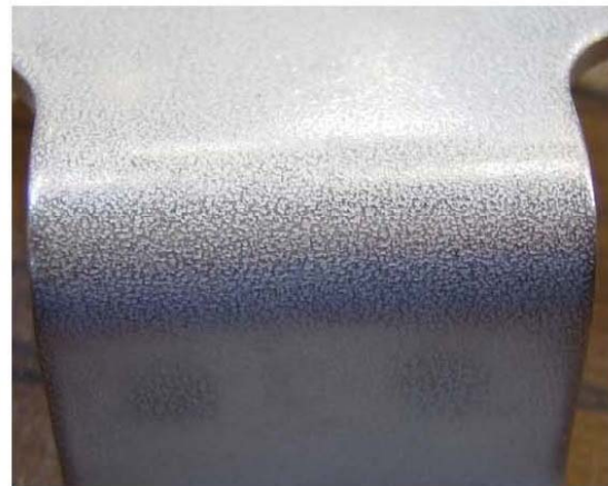
Nonconforming Pitted Surface (Discrepant Part)
